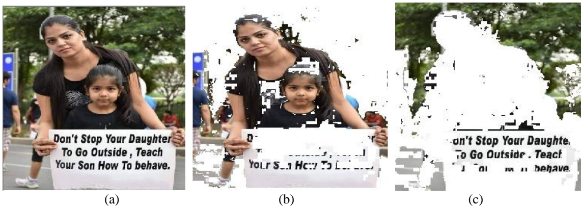
Figure 2. (a): Actual frame; (b): foreground separated frame; (c): background separated frame
