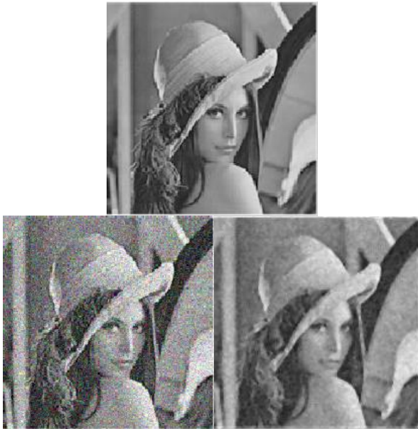
Figure 3. (a) Original image; (b) Image with Gaussian noise; (c) Image processed by Gaussian filter
