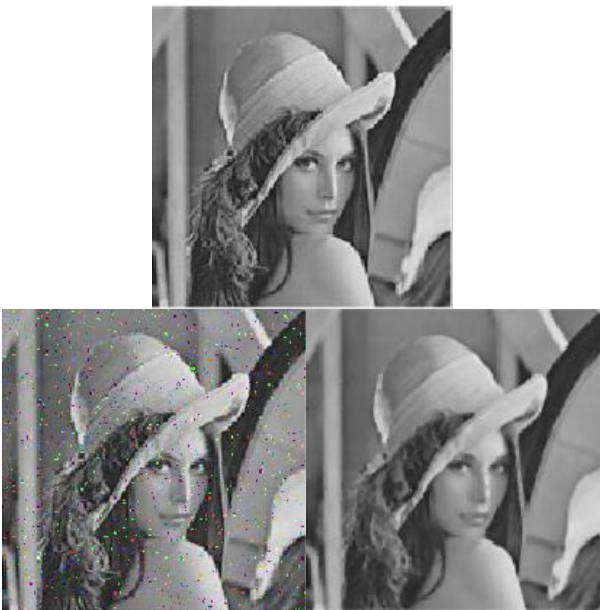
Figure 4. (a) Original image; (b) Image with salt-and-pepper noise; (c) Image processed by median filter
