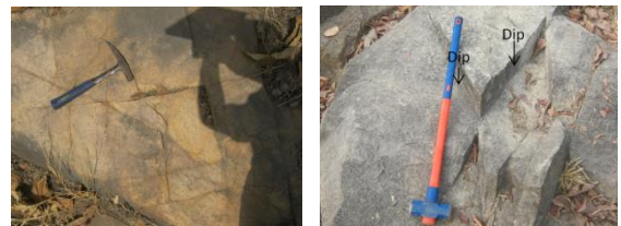
Figure 22. Photograph of major joints found on different rocks (A) Not dipping at (8° 43' 49.0" N and 8° 32' 07.2" E), (B) while dipping at (8° 43' 10.6" N and 8° 30' 07.6" E)
