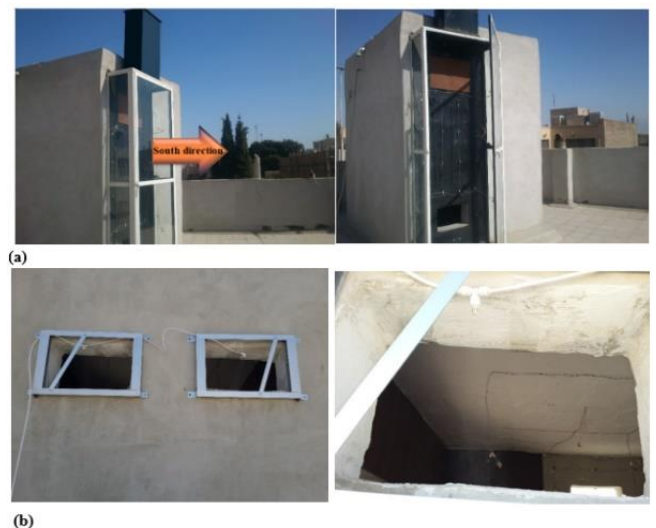
Figure 1. (a) Hybrid system configuration (b) water spraying system (WSS) at the back of the room [19]
