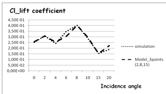
Figure 10a. Comparison of the lift coefficient of the simulation and our model
