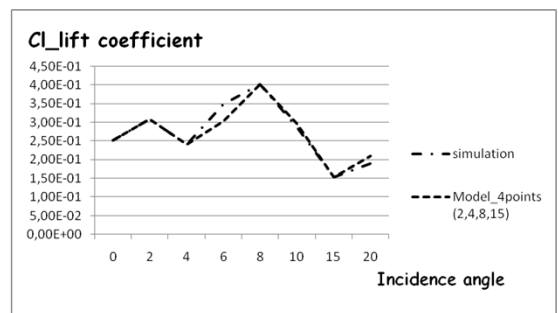
Figure 10b. Comparison of the lift coefficient of the simulation and our model
