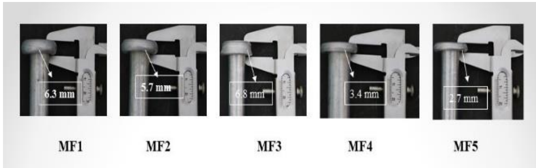
Figure 5. Measurement of flash width of mechtrode after friction surfacing
