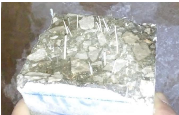
Figure 7. ARHP fibers after conservation of the concrete in a period of 365 days
