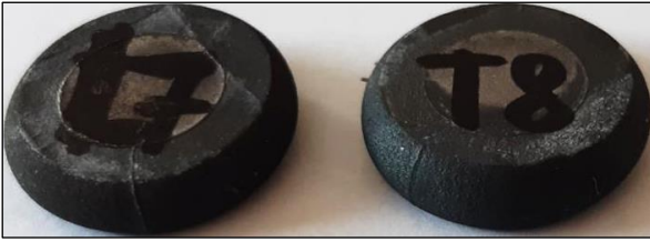
Figure 4. Photos of samples allow CrNi60WoTi after hot upsetting with deformation degree \sim 1.3 : T=1050^{\circ}\text{C} , U_c=10.0 \text{ sec}^{-1} , longitudinal and transverse (from left to right)
