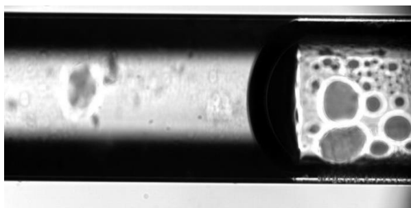
Figure 5. Transmission micrograph of a glass capillary (ID/OD = 300\mu\text{m}/400\mu\text{m} ) filled with water (left) and \text{CO}_2 (right) showing the difference of brightness due to reflection off the inner wall. Pressure: 10 MPa
