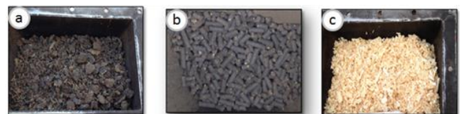
(a) Raw olive pomace, (b) Exhausted olive pomace, (c) Sawdust of wood
