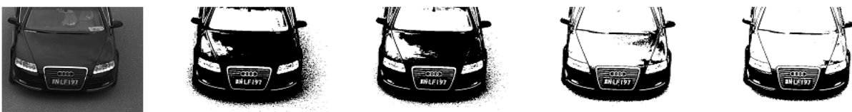
(1a) Original image; (1b) Result of Otsu's method; (1c) Result of graph cut algorithm; (1d) Result of our algorithm; (1e) Result of gold standard segmentation
