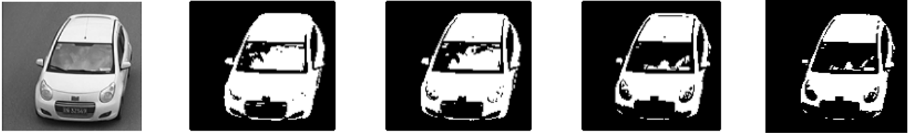
(3a) Original image; (3b) Result of Otsu's method; (3c) Result of graph cut algorithm; (3d) Result of our algorithm; (3e) Result of gold standard segmentation
