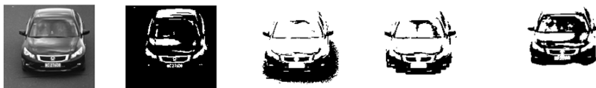
(1a) Original image; (1b) Result of Otsu's method; (1c) Result of graph cut algorithm; (1d) Result of our algorithm; (1e) Result of gold standard segmentation
