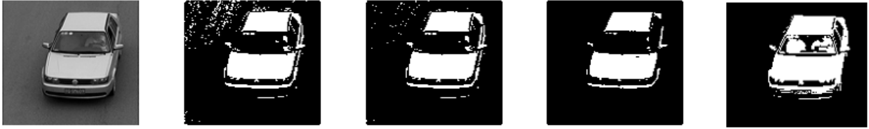
(2a) Original image; (2b) Result of Otsu's method; (2c) Result of graph cut algorithm; (2d) Result of our algorithm; (2e) Result of gold standard segmentation
