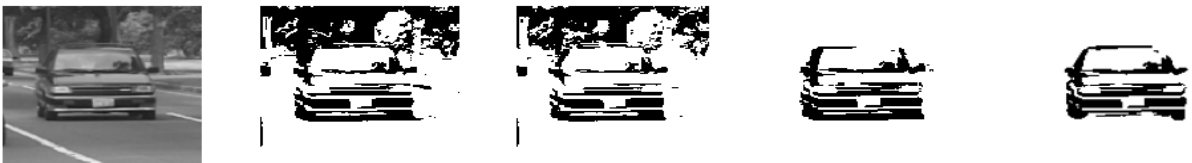
(3a) Original image; (3b) Result of Otsu's method; (3c) Result of graph cut algorithm; (3d) Result of our algorithm; (3e) Result of gold standard segmentation
