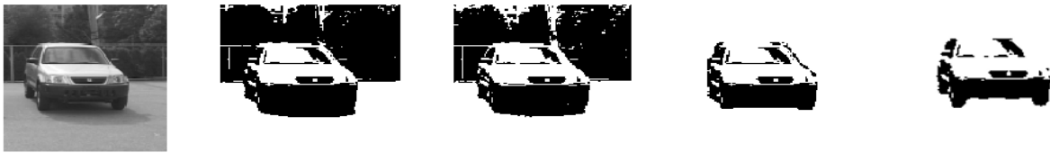
(1a) Original image; (1b) Result of Otsu's method; (1c) Result of graph cut algorithm; (1d) Result of our algorithm; (1e) Result of gold standard segmentation
