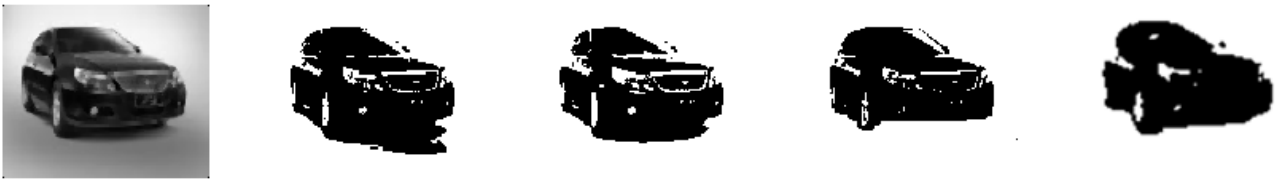
(4a) Original image; (4b) Result of Otsu's method; (4c) Result of graph cut algorithm; (4d) Result of our algorithm; (4e) Result of gold standard segmentation
