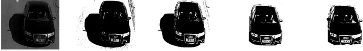
(3a) Original image; (3b) Result of Otsu's method; (3c) Result of graph cut algorithm; (3d) Result of our algorithm; (3e) Result of gold standard segmentation
