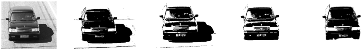
(2a) Original image; (2b) Result of Otsu's method; (2c) Result of graph cut algorithm; (2d) Result of our algorithm; (2e) Result of gold standard segmentation
