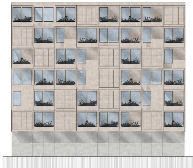
Figure 6. Facade of the apartment building with a possible combination of the interchangeable balcony units
