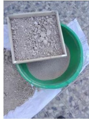
(A) Sand of type was brought from east of Jordan and was sieved with a sieve No. 1
