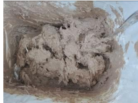
(B) The straw was mixed with soil and water was added as needed
