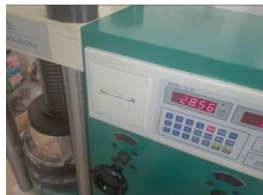
Figure 4. The strength of bricks is 28.56 Kn/m 2
