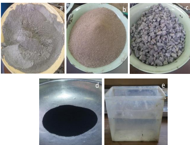
Figure 1. Samples of (a) cement, (b) sand, (c) granite, (d) crumb; and (e) water used for concrete
