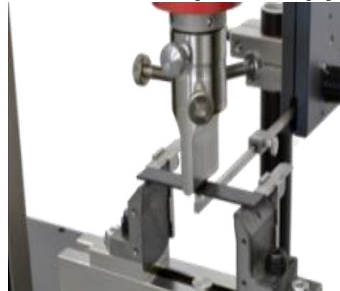
3(b) Flexural test equipment
