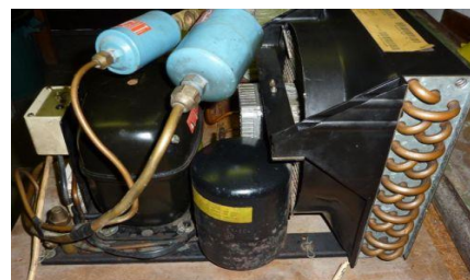
Figure 2. Danfoss SC15BXT2 compressor installation
