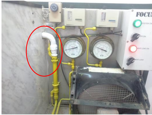
Figure 6. Illustrative picture, indicating the amount of the accumulated ice on one part of the refrigeration circuit
