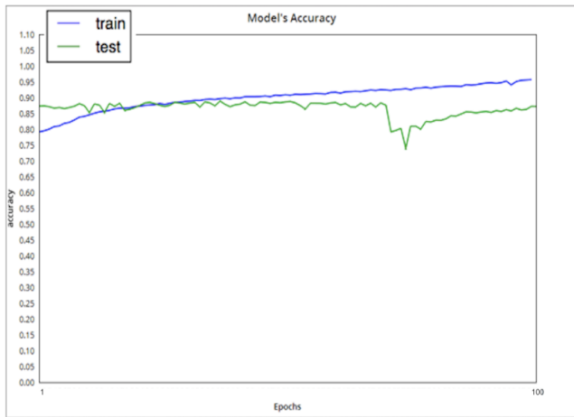
Figure 4. Accuracy for 100 epochs of training with three convolutional layers and SGD optimizer on the first version of the dataset
