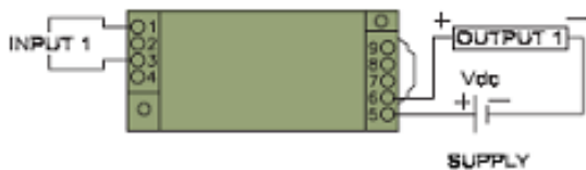
Figure 4. Wiring schematic of Voltage transducers
