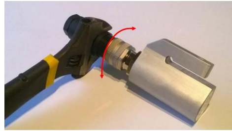
Figure 9. Rail temperature sensors
