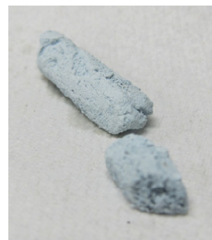
Figure 2. Spent anode exhibiting clay-like morphology
