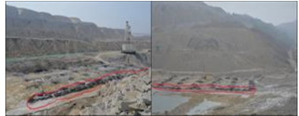
Figure 2. Blasting face with line drilled blastholes at Jayant opencast project
