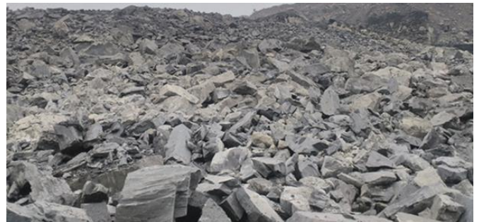
Figure 14. Over view of fragmentation resulted due to blasting at Dragline bench of East section of Jayant Opencast Project
