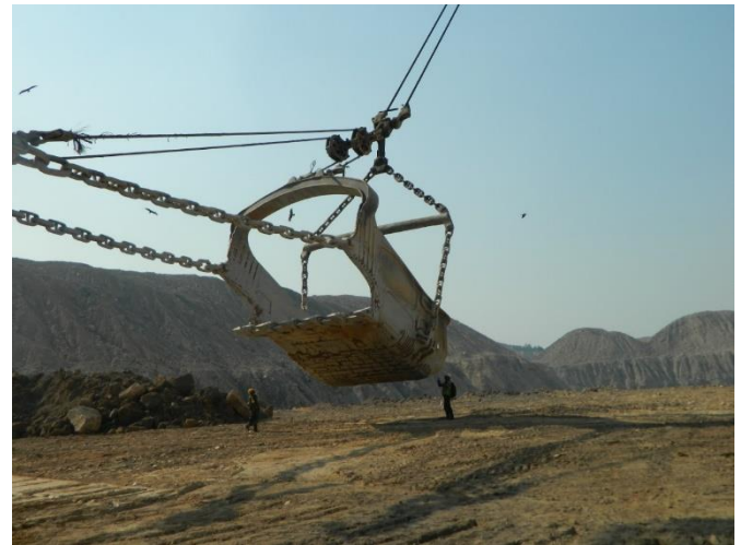
Figure 1. A dragline bucket (62m 3 )
