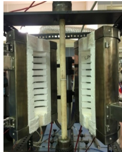
Figure 4. c Close view of Experimental Set-up with anode and cathode compartments and Single SOFC cell assembly at the center
