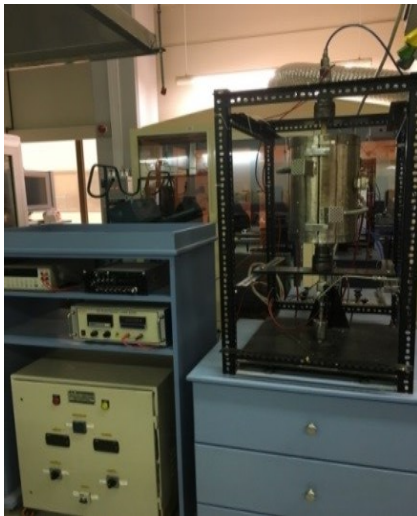
Figure 4. b Experimental Set-up for testing 16mm dia single SOFC cells
