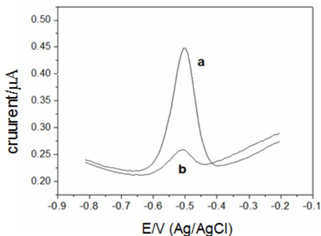
Figure 3. DPV response of the aptasensor in the prepared solution containing 0.6 mL of  $10^{-6}$  mol/L P1 (b) in the presence of thrombin ( $c = 2.6 \times 10^{-9}$  M) (b) without thrombin.
