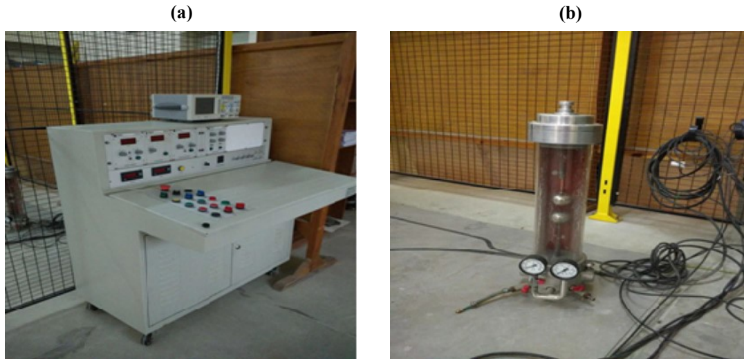
Figure 3. Test equipment used: (a) Control and measurement unit; (b) Testing vessel (HV-9134) for AC setup.
