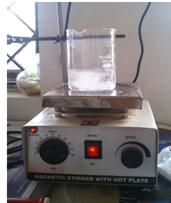
Figure 5. Magnetic stirring of MgO based nanofluid mixture
