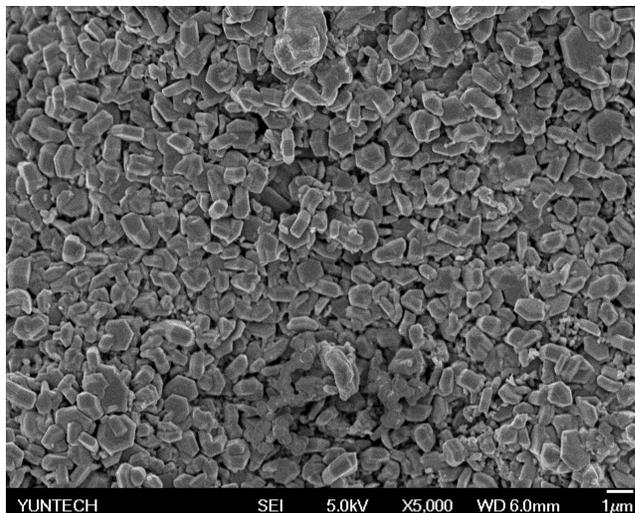
Figure 8. The SEM image of the ZnS film on top of the CuInS<sub>2</sub> layer
