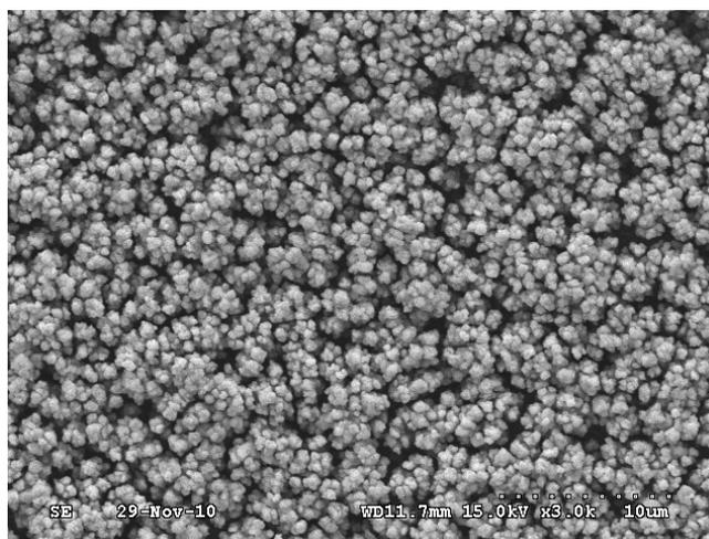
Figure 3. The SEM image of the Cu-In film on top of Mo glass
