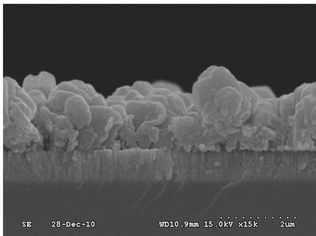
Figure 10. The cross-section of the CIS solar cell.
