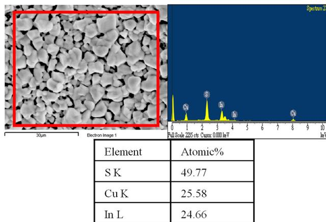
Figure 5. The EDS composition of the CuInS<sub>2</sub> film
