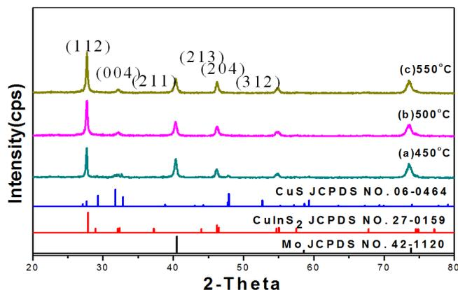
Figure 4. The XRD of the film after sulfurization
