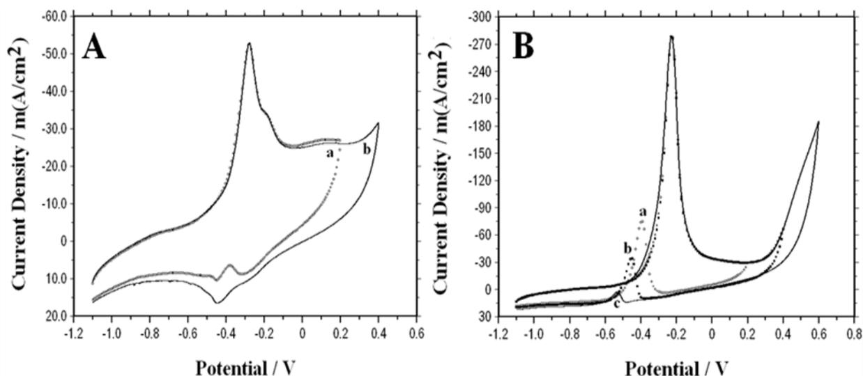
Figure 7. CVs of OMO/Pd modified electrooxidations of (A) methanol (1M CH<sub>3</sub>OH/ 1M KOH) in the scanning potential regions of (a) -1.1 to +0.2 , (b) -1.1 to +0.4 and (B) EG (1M EG / 1 M KOH) in the scanning potentials at (a) -1.1 to +0.2 , (b) -1.1 to +0.4 and (c) -1.1 to +0.6 V [scan rate 50 mV/s]
