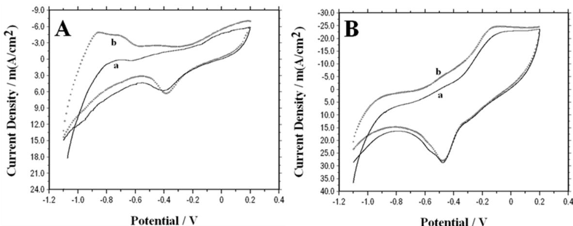
Figure 4. (A) Cyclic voltammograms of C/Pd and (B) OMO/Pd modified electrode at the (a) first and (b) fourth cycle in 1M KOH at 50mV/s
