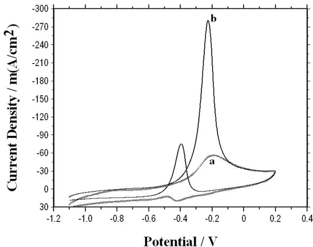
Figure 6. CVs of OMO/Pd modified electrode in 1M EG / 1M KOH (a) 4<sup>th</sup> and (c) 18<sup>th</sup> cycle [Scan rate 50 mV/s]
