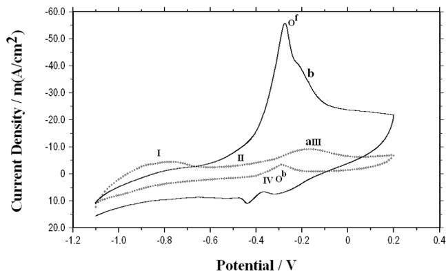
Figure 5. CVs of (a) Pd/OMO electrode in 1M KOH and electrooxidation of 1M CH<sub>3</sub>OH in (b) C/Pd and (c) OMO/Pd modified electrode in 1 M KOH [Scan rate 50 mV/s].
