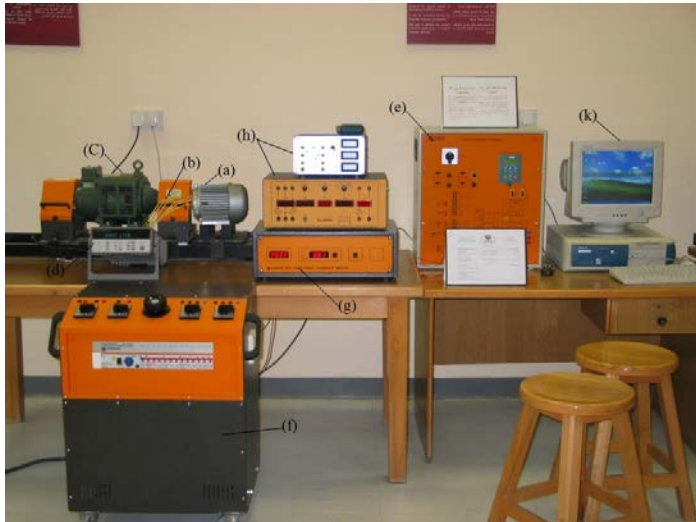
Figure 12- experimental setup used for validating the thermal model of JLEM three phase 1.5 kW induction motor.
