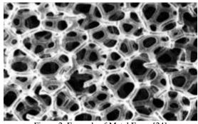
Figure.2. Example of Metal Foam [24]
