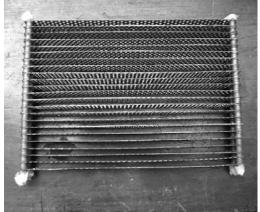
Figure.1. photograph of porous heat exchanger sample [14]
