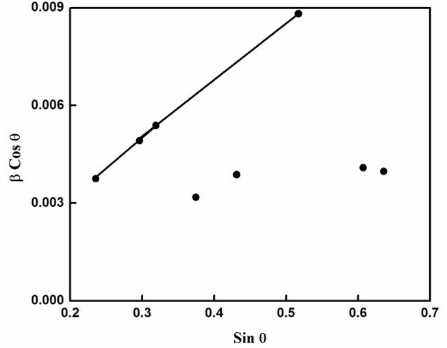
Figure 4. Williamson Hall plot of  $\text{Cu}_2\text{Te}$  thin film electrodeposited on  $\text{SnO}_2:\text{F}$  substrate at bath temperature  $80^\circ\text{C}$ .
