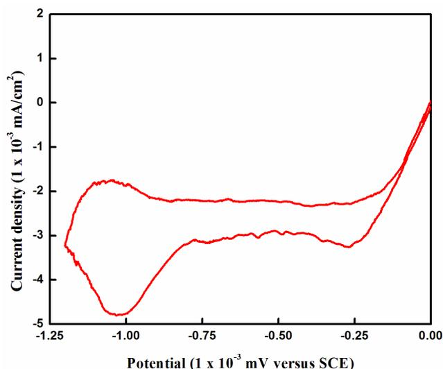
Figure 1. Cyclic voltammogram recorded for  $\text{Cu}_2\text{Te}$  thin films obtained on  $\text{SnO}_2:\text{F}$  substrate from an electrolytic bath consists of  $\text{CuSO}_4$  and  $\text{TeO}_2$ .
