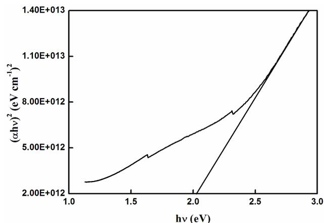
Figure 5. Plot of  $(\alpha hv)$  versus  $(\alpha hv)^2$  for  $\text{Cu}_2\text{Te}$  thin film electrodeposited on  $\text{SnO}_2:\text{F}$  substrate at bath temperature  $80^\circ\text{C}$ .
