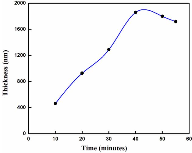
Figure 2. Variation of film thickness with deposition time for  $\text{Cu}_2\text{Te}$  thin films obtained on  $\text{SnO}_2:\text{F}$  substrate.
