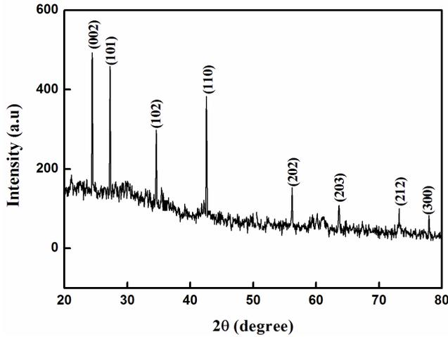
Figure 3. X-ray diffraction pattern recorded for  $\text{Cu}_2\text{Te}$  thin films obtained on  $\text{SnO}_2:\text{F}$  substrate at bath temperature  $80^\circ\text{C}$ .
