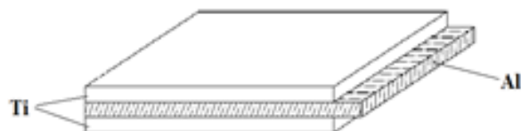
Figure 1. The model of Ti-Al laminated composite material sample
