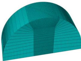
Figure 2. The computational mesh model of the workpiece
