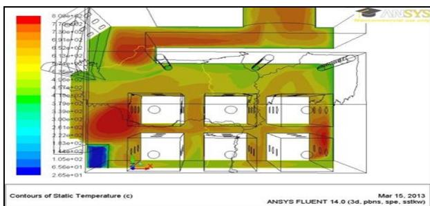
**Figure 7.** Validation cat. 4, temperature contour at the central plane
