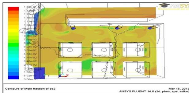
**Figure 11.** Validation cat. 4,  $CO_2$  contour at the central plane
