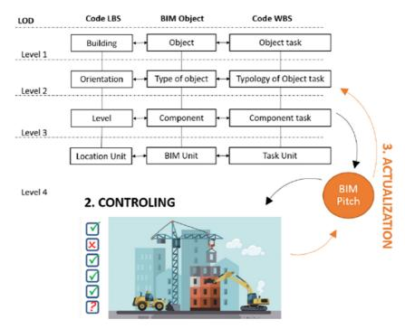
Figure 1: The concept of the proposed BIM framework.
