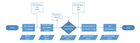
Figure 4: The BIM framework process.
