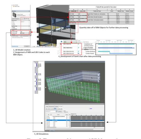
Figure 5: The process of the proposed BIM framework.
