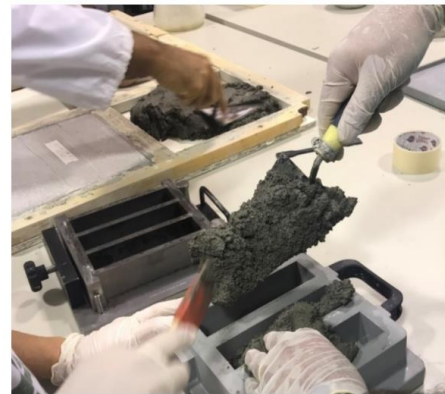
Figure 5. The mixture is poured into the formworks
