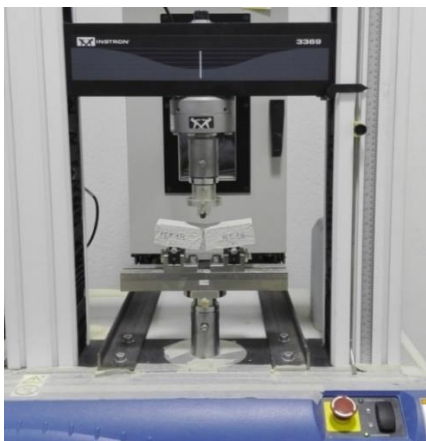
Figure 6. Specimen during a three point flexural test
