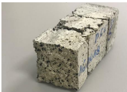
Figure 7. PVC 20 specimen after compressive test
