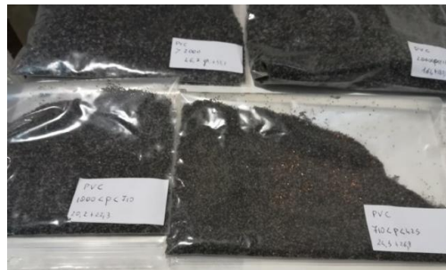
Figure 3. PVC-Cu sieving results; on the right the presence of copper in particle size up to 710 mm is observable
