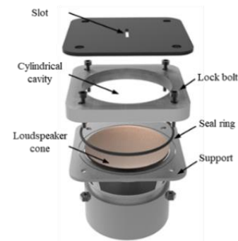
Figure 3. The synthetic jet actuator
