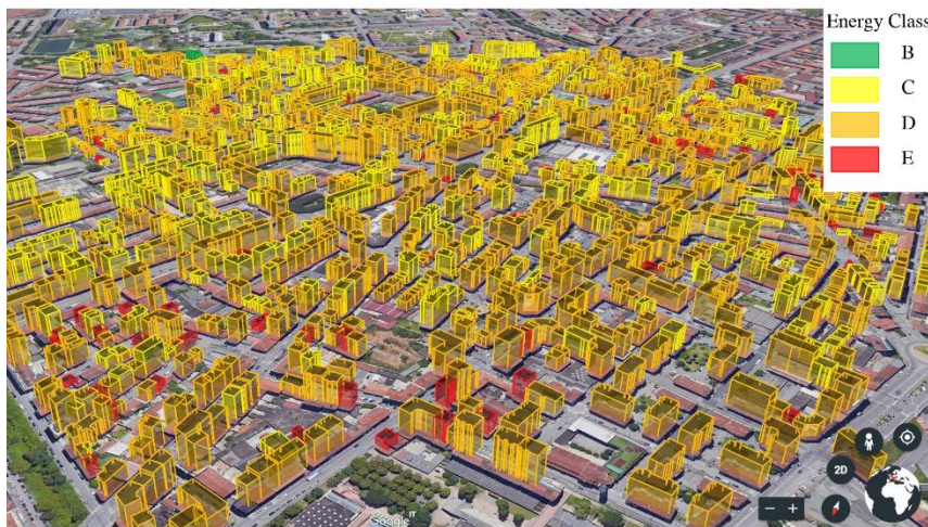
Figure 14. Energy class from the application of the annual space heating and domestic hot water models
