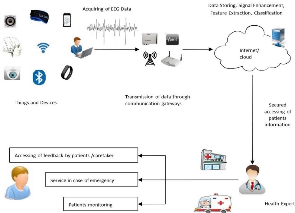
**Figure 1.** Proposed model of cloud based health IoT system for epileptic patient monitoring
