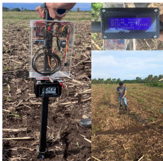
Figure 6. Field installation of the Internet of Things (IoT)-based electrical conductivity (EC) measurement system
