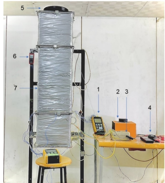
Figure 1. Photograph of the experimental setup, (1) digital thermocouple thermometer, (2) Variac, (3) digital power meter, (4) digital anemometer, (5) exhaust fan, (6) digital differential pressure meter, and (7) heated test section
