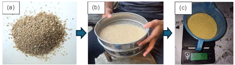
Figure 3. Preparation of the quartz sand bed material (adapted from Winaya et al. [17]), (a) raw silica sand, (b) sieving to obtain a uniform particle size, and (c) weighing prior to loading into the reactor
