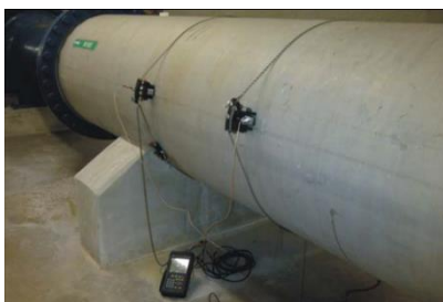
Figure 1. Arrangement of the ultrasonic flowmeter in the hydraulic method
