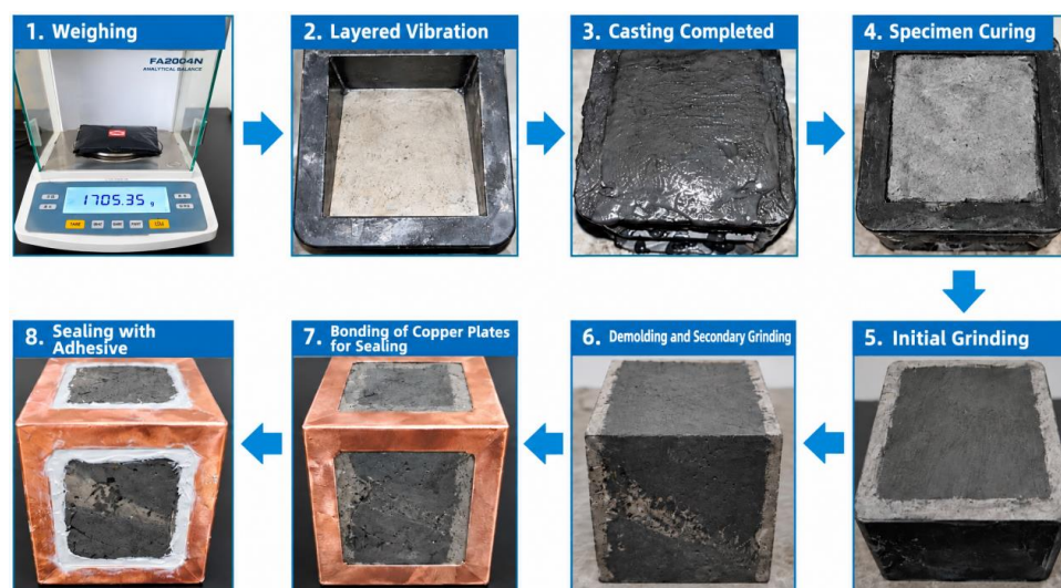
Figure 3. Specimen preparation procedure
