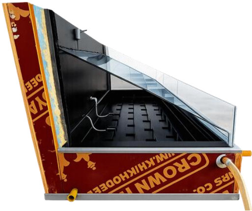
Figure 9. The installation of the south-facing fins in the double-basin solar still (DBSS)
