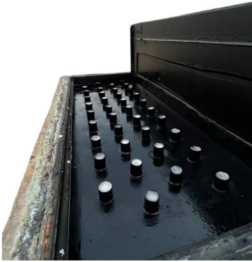
Figure 11. Installation of the phase change material (PCM)-hollow cylindrical fin in the double-basin solar still (DBSS) lower basin
