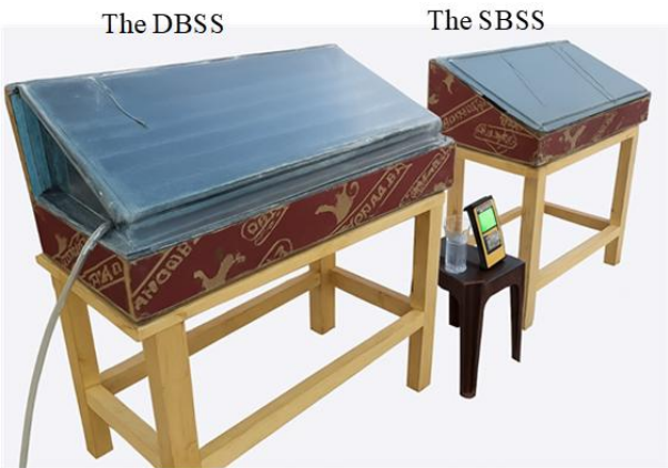
Figure 6. The installation of the single-basin solar still (SBSS) and the double-basin solar still (DBSS)
