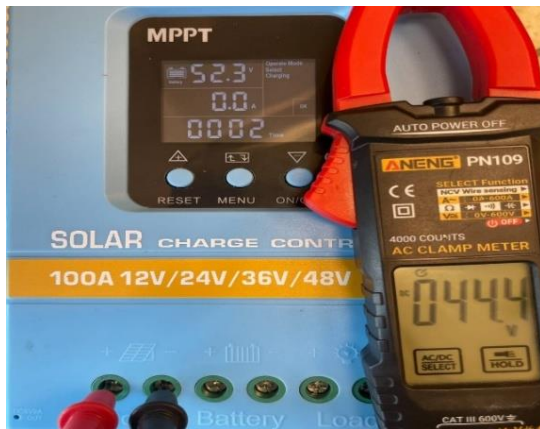
Figure 15. Measured direct-current (DC)-link voltage of the photovoltaic (PV)/LiFePO 4 -battery-supported source
