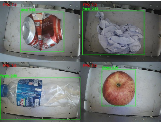
Figure 17. Waste detection results on RP5 using the YOLOv8n model
