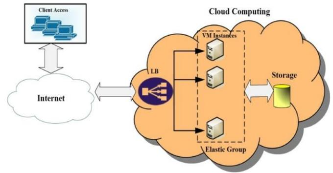
Figure 1. Web application hosting architecture
