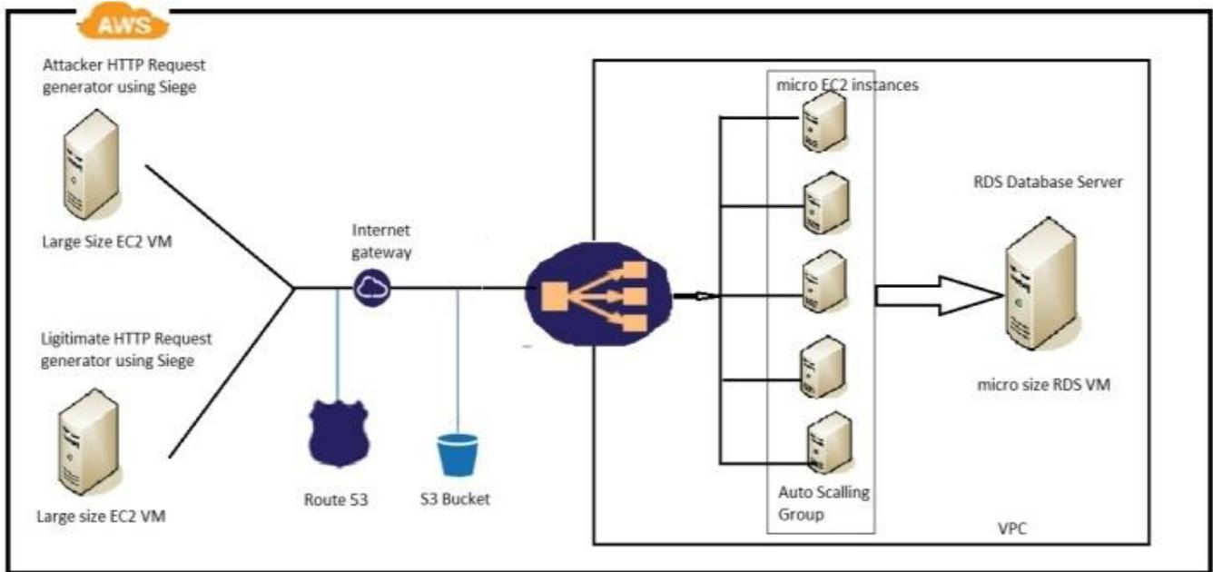
Figure 3. Experimental test-bed for hosting web application in the Amazon AWS
