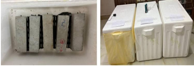
Figure 2. The controlled environmental chambers designed to maintain the specified temperature and humidity levels
