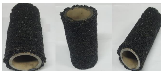
Figure 2. The carbon steel oil pipe with the protective composite shield
