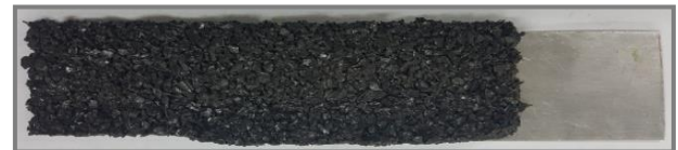
Figure 7. The tensile strength test sample for the adhesion power between the protective composite shield and the pipe
