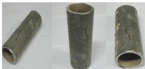
Figure 1. The carbon steel oil pipe without the protective composite shield
