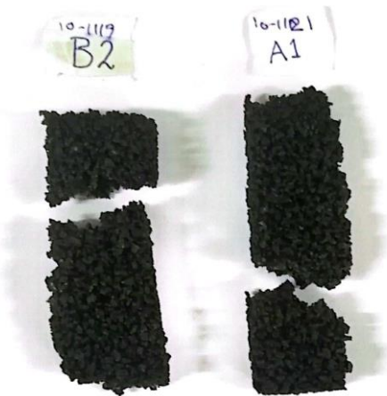
Figure 6. Representative fractured specimens after tensile testing (B2 and A1)
