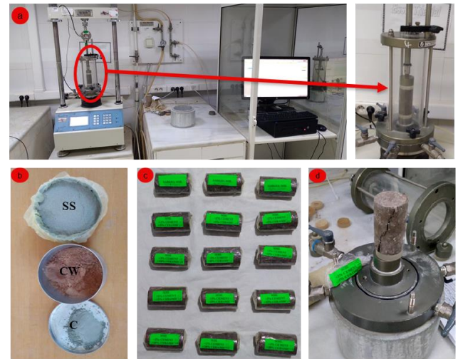
Figure 6. Unconfined compressive strength (UCS) test apparatus: (a) axial loading machine, (b) materials, (c) samples before testing, and (d) sample after testing
