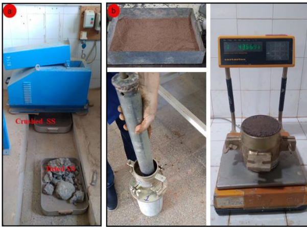
Figure 5. (a) Crush machine and (b) Proctor test apparatus
